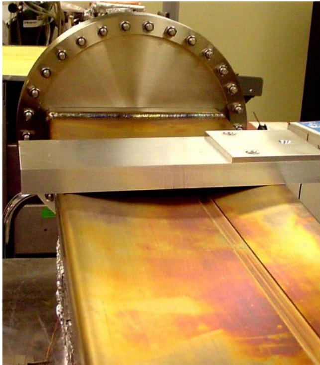
*Distorted copper chamber during a bakeout*
